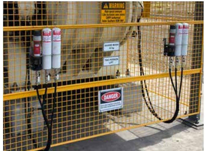
**Application** Conveyor pulley bearings and seals
