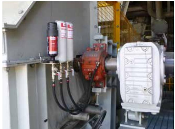
**Application** Conveyor pulley bearing and seal
