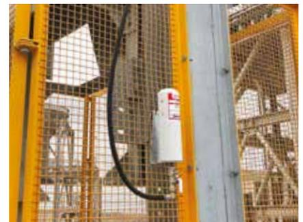
**Strategy 3** – Remote mount lubricators used for conveyor pulley bearings which are located behind cages and avoid unnecessary manual handling of cages.
