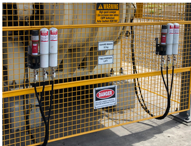
Application Conveyor pulley bearings and seals Lubricator perma STAR VARIO 500 cm³ Installation kit 2 x K3CHCX
