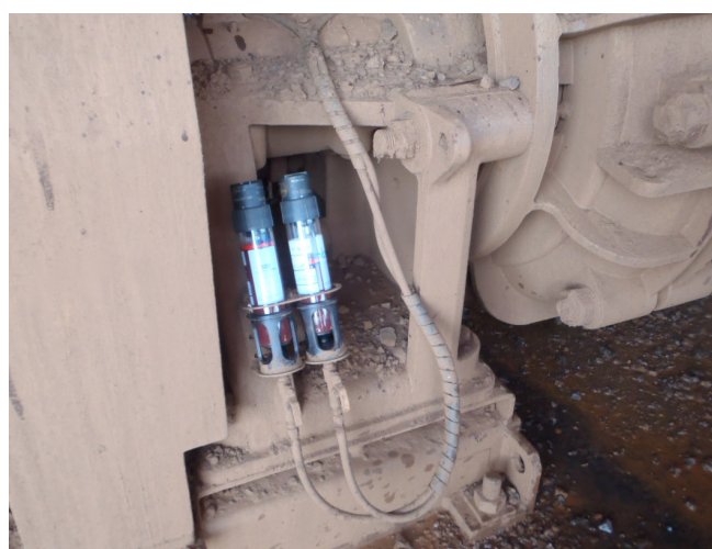
Application Labyrinth seals Lubricator perma STAR VARIO 500 cm 3 Installation kit K265CX
