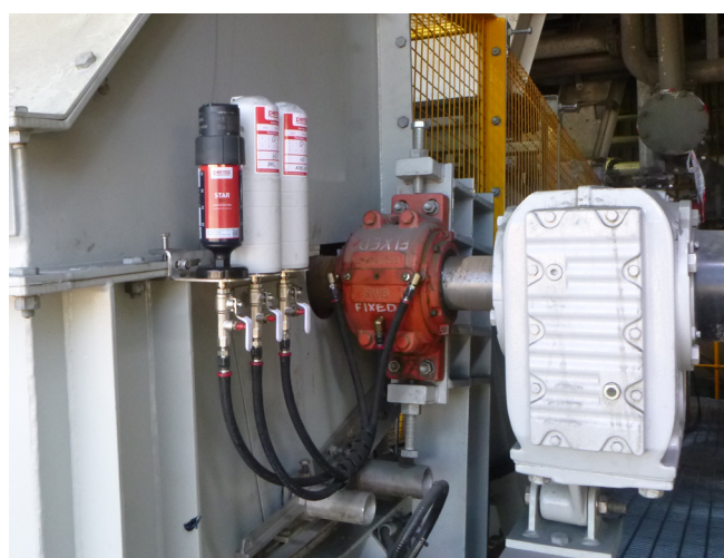
Application Conveyor pulley bearing and seal Lubricator perma STAR VARIO 250 cm³ Installation kit K330
