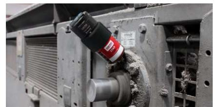
Lubrication of flange bearing on a conveyor
