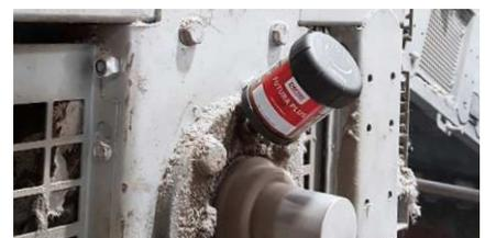
Lubrication of flange bearing on a conveyor
